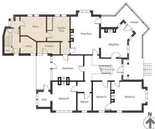
Figure 2.27 Ground Floor Plan in 2012. The 1950s alterations and additions to Sunny Brae are shown shaded. Source: David White Architects, 2020.
