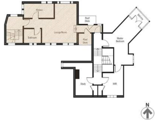
Figure 2.28 Upper Floor plan in 2012. The 1950s alterations and additions to Sunny Brae are shown shaded. Source: David White Architects, 2020.
