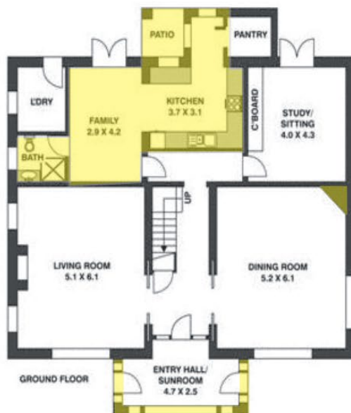
Figure 2.47 Changes to the existing building at 53 Drumalbyn Road, Lower level floor. Source: www.realestate.com.au
