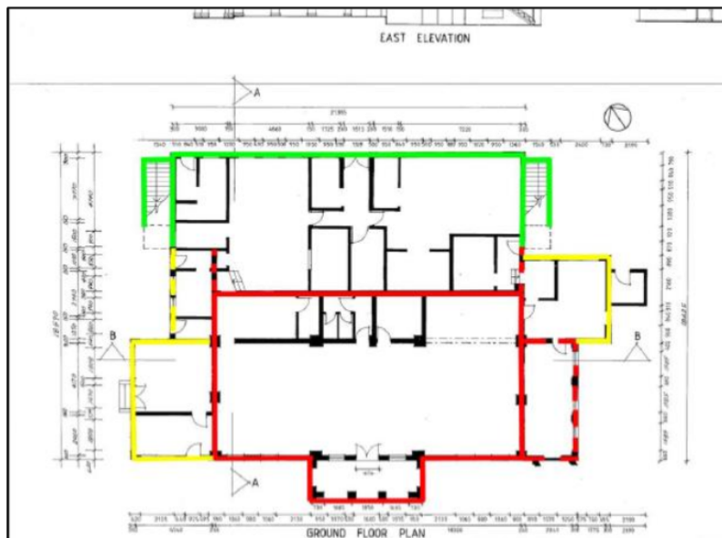
Figure 2. 'Significant elements of the George S. Grimley Pavilion' – areas of high significance have been coloured in red, moderate significance in yellow and little significance in green. The first floor of the building is identified as having high significance. Source: Woollahra Council, annotations by WP Heritage and Planning.
