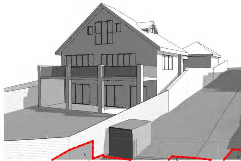
4 PROPOSED ELEVATIONAL SHADOW DIAGRAM - 12PM 21 JUN Additional shadow due to development
