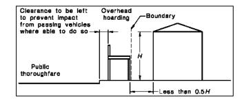
The Principal Contractor or Owner-builder must ensure that overhead protective structures are installed and maintained in accordance with the NSW "Code of Practice - Overhead Protective Structures 1995". This is code available at <a href="https://www.safework.nsw.gov.au/">www.safework.nsw.gov.au/</a> data/assets/pdf\_file/0008/52883/Overhead-protective-
